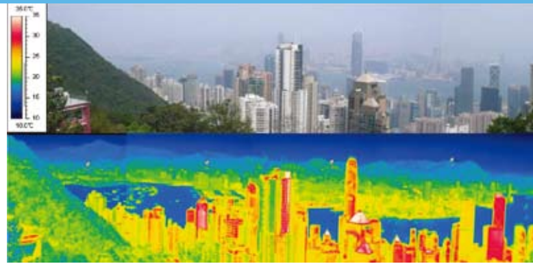
An infrared photo of the surface temperature profiles of Hong Kong on 15 March 2008 16:00. The color scale indicates the surface temperature. It can be seen that some building surfaces are much warmer than others. We suggest that the warmer building and mountain surfaces than ambient air create upward buoyancy flows to drive natural ventilation of the city.
